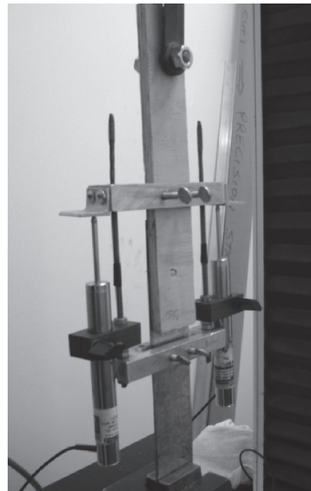
Figure 5: Small element lateral strength (shear) tests
