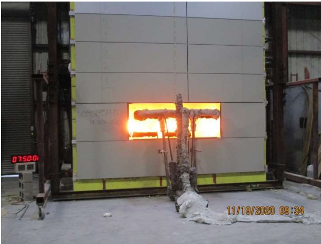
Commencement of Phase 2 NFPA 285 Test
