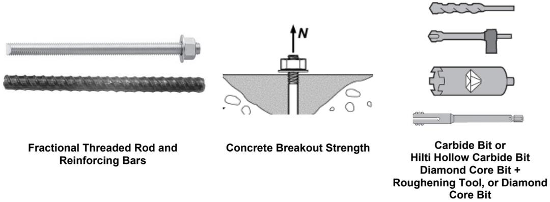
**TABLE 7—CONCRETE BREAKOUT DESIGN INFORMATION FOR FRACTIONAL THREADED ROD AND REINFORCING BARS ALL DRILLING METHODS<sup>1</sup>**
