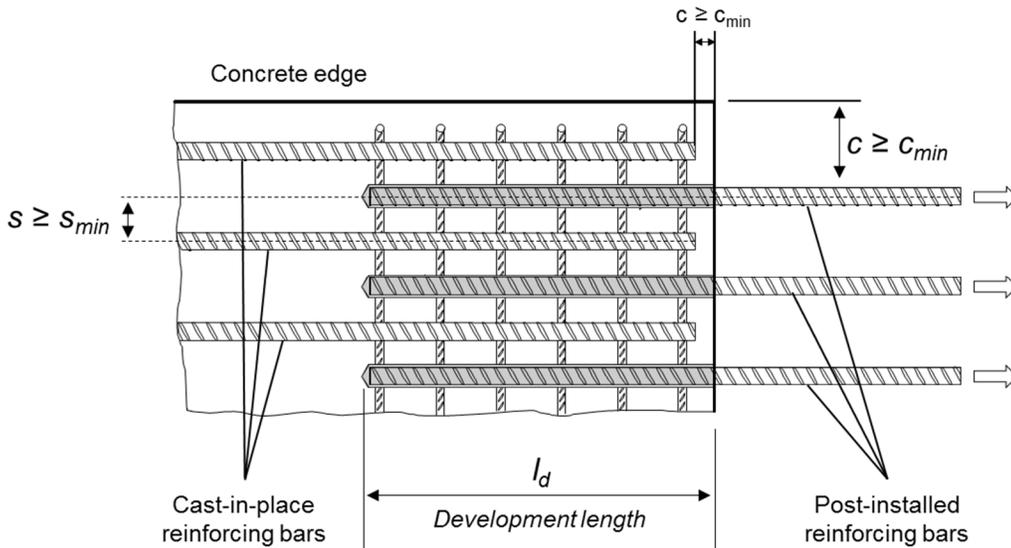
FIGURE 2—INSTALLATION PARAMETERS FOR POST-INSTALLED REINFORCING BARS
