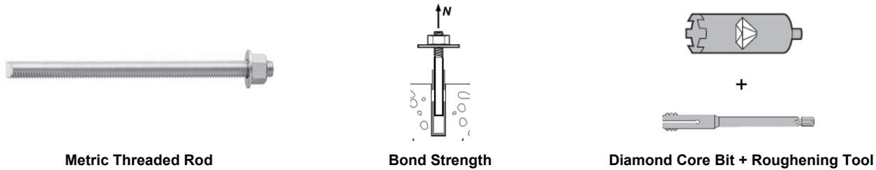
**TABLE 20—BOND STRENGTH DESIGN INFORMATION FOR METRIC THREADED RODS IN HOLES CORE DRILLED WITH A DIAMOND CORE BIT AND ROUGHENED WITH A HILTI ROUGHENING TOOL<sup>1</sup>**
